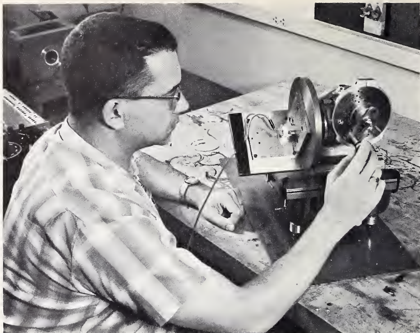
This NBS device provides highly accurate and reproducible calibrations of acceleration to 1 g by reference to earth's gravitational field.
