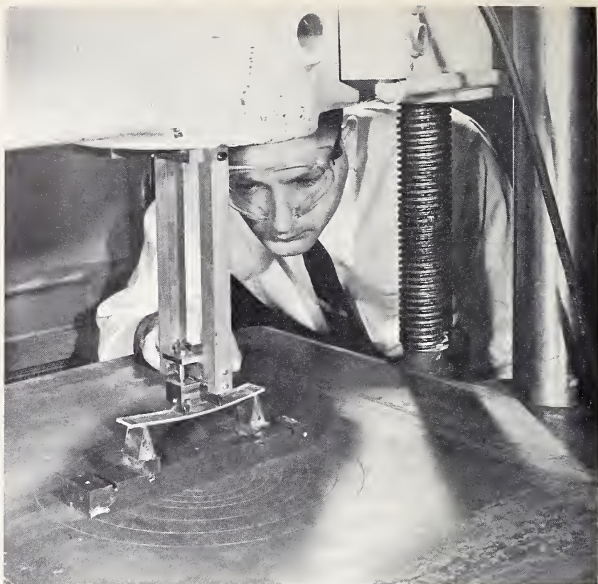
Examination of a specimen of chemically strengthened glass that is undergoing a rupture test.
