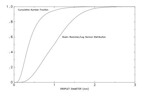
Figure 3.4: Cumulative Volume Fraction and Cumulative Number Fraction functions of the droplet size distribution from a typical industrial-scale sprinkler. The median diameter  $d_m$  is 1 mm,  $\sigma = 0.6$  and  $\gamma = 2.4$ .
