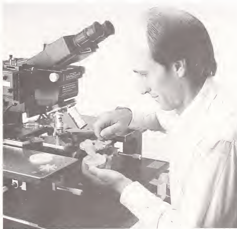
NIST electrical engineer Dylan Williams examines a microwave chip at one of NIST's wafer probe workstations.
