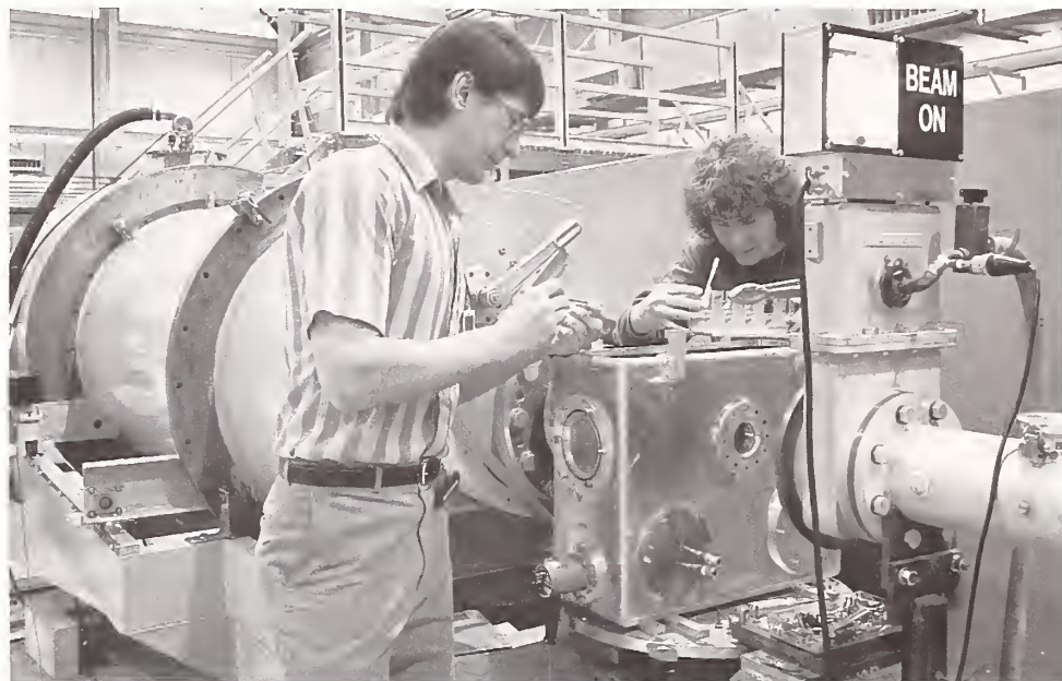
Research physicists John Barker (left) and Susan Krueger insert a sample into NIST's 8-meter small-angle neutron scattering spectrometer at the NIST Cold Neutron Research Facility, a national user facility for materials research.
