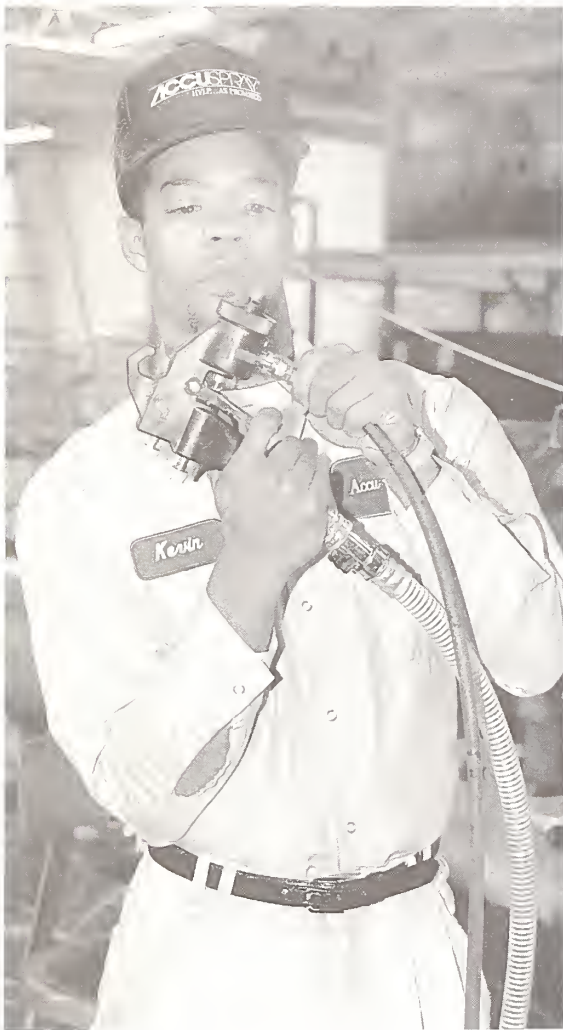
The Great Lakes Manufacturing Technology Center helped AccuSpray Inc. redesign its product and production method. Here, an AccuSpray employee demonstrates the special paint spraying equipment, which uses half the paint of conventional methods.
