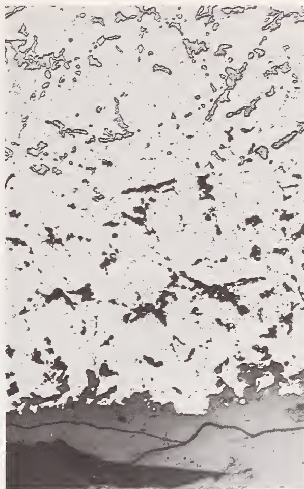
FIGURE 3. High mercury content amalgam after four months exposure to 1 percent NaCl solution.
