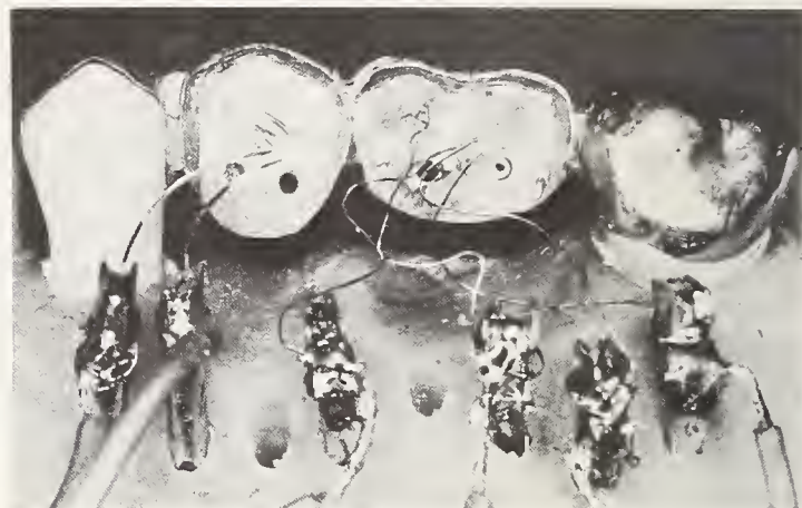
FIGURE 2. Foil strain gages attached to a four-unit gold alloy posterior bridge.
