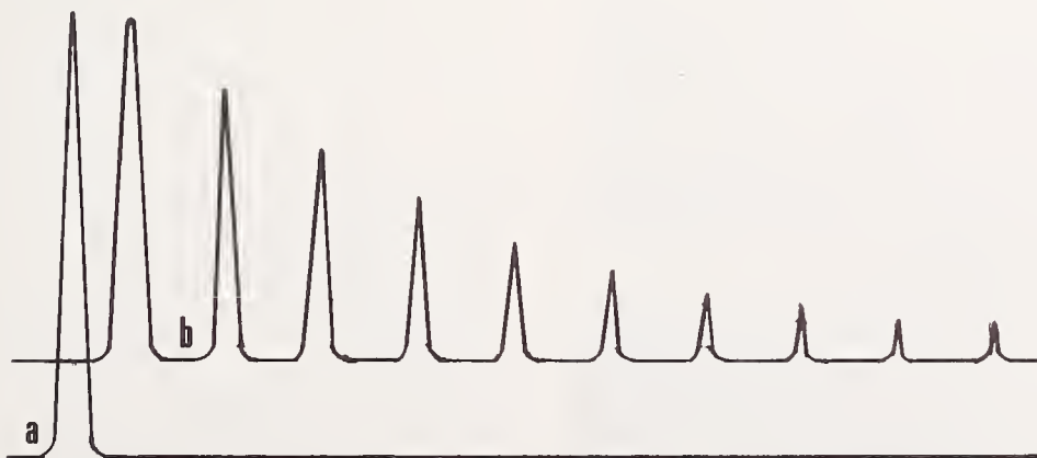
FIGURE 5. Pulse echo pattern, a—input pulse, b—pulses after passage through specimen.
