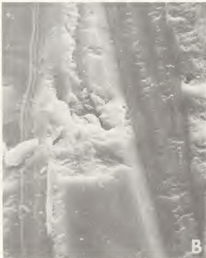
FIGURE 6. Bovine enamel polished with various abrasives (Magnification 9000 \times ). A: 220 grit paper ; B: 440 grit paper ; C: 600 grit paper ; D: \gamma -alumina.
