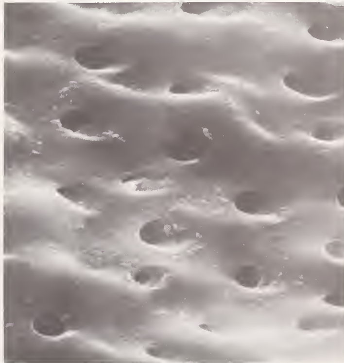
FIGURE 9. Bovine dentin treated with 50 percent aqueous formic acid for one minute (Magnification: 3000X).
