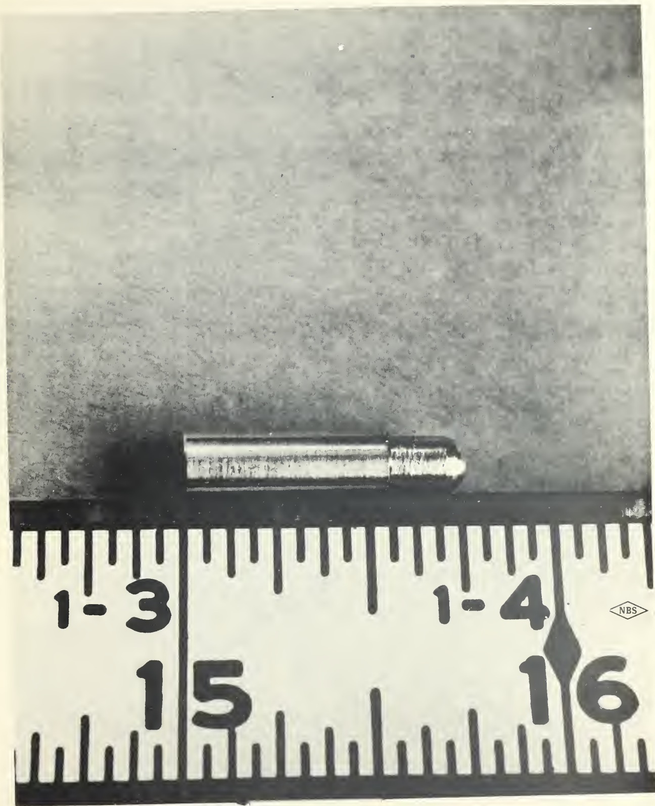
Figure 1. Sievert ionization chamber, showing small size.
