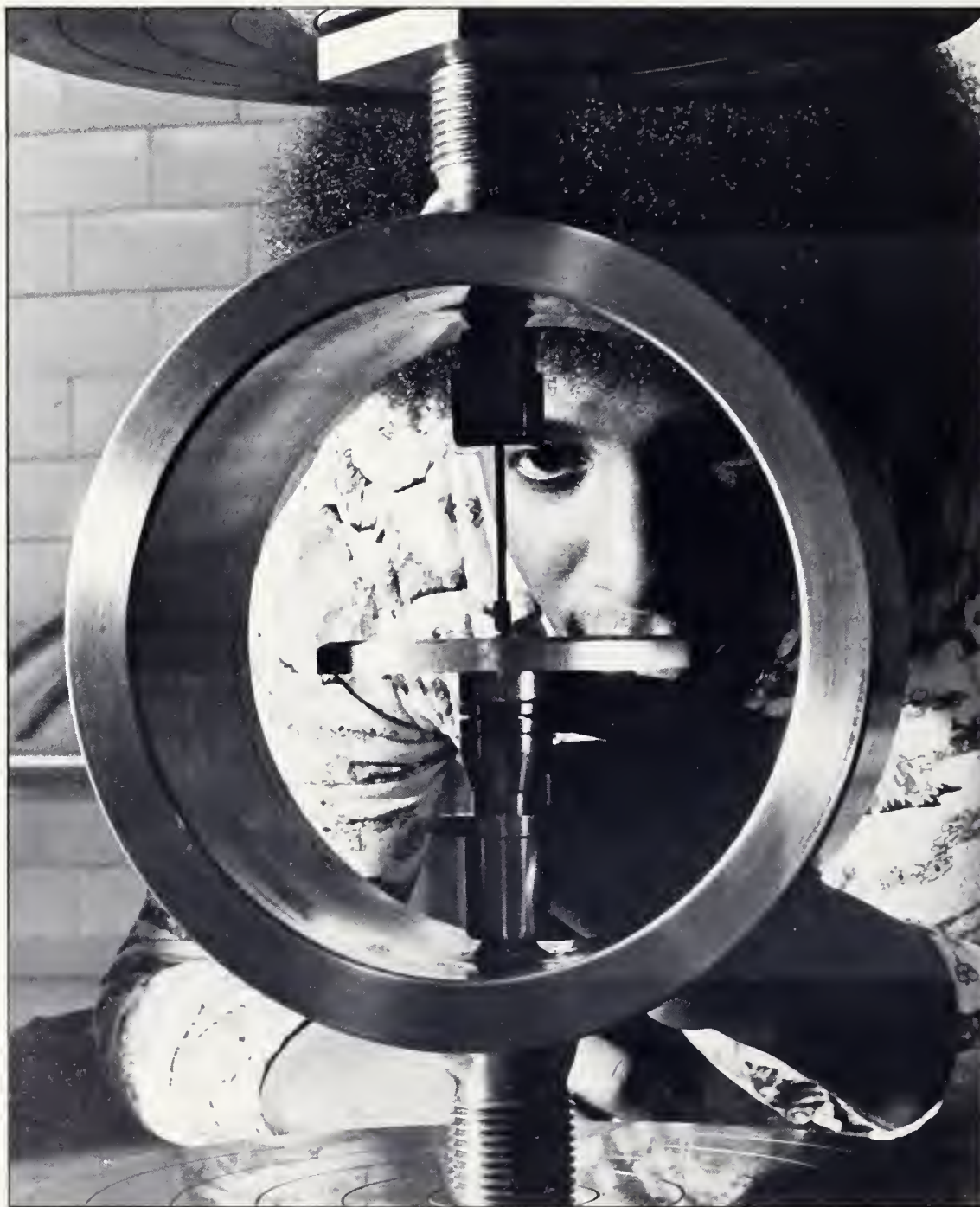
NBS proving ring used for calibration services.
