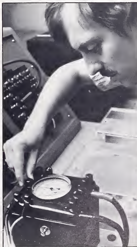
Calibrating watt-hour meters.
