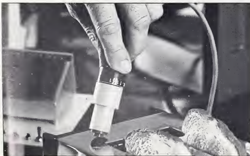
NBS-developed device measures burn potential of appliances
