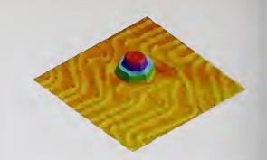
Figure 6. Scanning tunneling microscope image  $(32 \text{ nm} \times 32 \text{ nm})$  of a 9 nm mound, two atomic layers high, created by the impact of a single Xe<sup>44+</sup> ion on the Au(111) surface. The mound has relaxed to a perfect hexagon, and the "herring-bone" reconstruction in the back-ground has rearranged around the mound to minimize surface energy.
