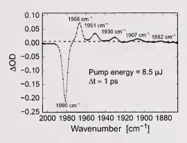
Figure 4. Spectrum showing differential absorption for vibrationally excited  $W(CO)_6$  in room-temperature *n*-hexane as a function of probe frequency. A strong ground-state bleach signal at 1980 cm<sup>-1</sup> is accompanied by five new absorption bands, from the first five  $v + 1 \leftarrow v$  hotband transitions.
