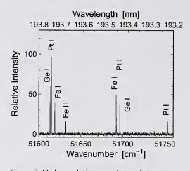
Figure 7. High-resolution spectrum of iron, germanium, and platinum, showing lines measured as wavelength standards for lithography at 193 nm.
