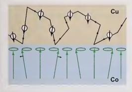
Figure 4. Electron diffusing near a ferromagnetic interface. The spin of the electron diffusing in the copper has its direction changed when it scatters from a cobalt interface with an in-plane spin wave.
