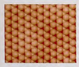
Figure 1. Binding site image for a cobalt atom on a copper (111) surface, showing three-fold symmetry.
