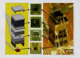
Figure 6. Photomicrograph of the physics package of a NIST chip-scale atomic clock, with a schematic diagram.
