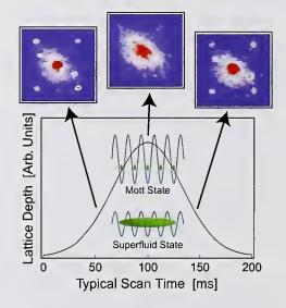
Figure 3. As the 3-D lattice depth is increased, the tunneling between lattice sites decreases. At a lattice depth of around 10 recoil energies, the system undergoes the Mott transition, and the diffraction pattern disappears. The transition is reversible, and the diffraction reappears when the lattice depth is reduced.
