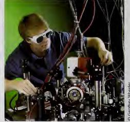
Figure 2. The calcium-atom optical frequency standard, being adjusted by Chris Oates.
