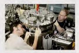
Figure 7. James Fedchak and Allan Smith install the new 10 cm collimator in the LBIR Facility to reduce the uncertainty in the calibration of the BXR I transfer-standard radiometer.
