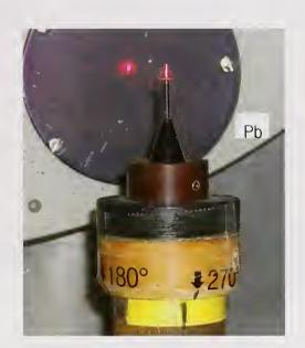
Figure 6. Close-up view of a seed (illuminated by a laser), mounted vertically on a rotating post, ready for calibration on the WAFAC calibration range.
