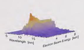
Figure 9. EUV spectra of xenon, taken on the NIST EBIT. The variation of spectral features as a function of the electron beam energy provides valuable data for benchmarking models of the atomic processes.
