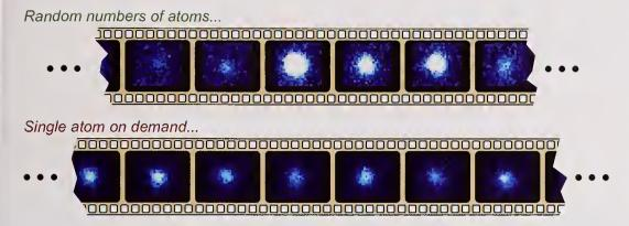
Figure 9. Real-time images of single atoms in an atom-on-demand source. Without feedback, the number of atoms is random, fluctuating between one, two, and three. With feedback, there is always just a single atom in the source.
