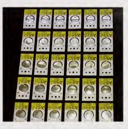
Figure 2. Radioactive test sources developed at NIST for the testing and evaluation of radiation detectors to be used by first responders.
