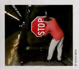
Figure 6. Cameron Miller mounts a STOP sign on the goniometer at the NIST Center for High-Accuracy Retroreflection Measurements (CHARM).
