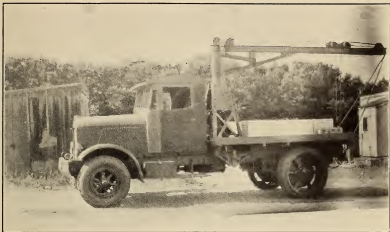
FIGURE 9.—General view of large-capacity scale-testing equipment of Suffolk County, N. Y.
