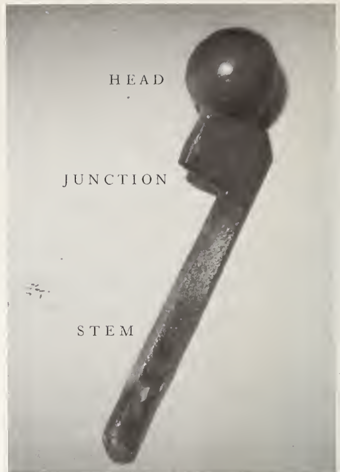
FIGURE 6. A prosthetic femoral head replacement for a Rhesus monkey is labeled to show the three segments of the device.
