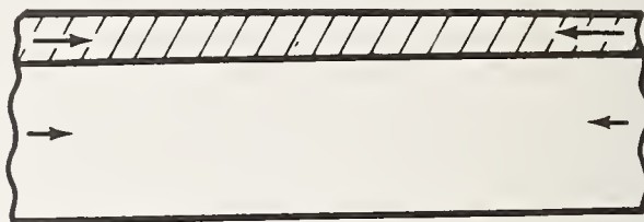
FIGURE 3. Development of interfacial stresses between a flame spray coating and a prosthesis due to thermal expansion mismatch.
