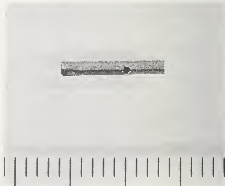
FIGURE 2. Porous tube having two diametrically opposite longitudinal micro-slots made by a spark discharge machining technique.
