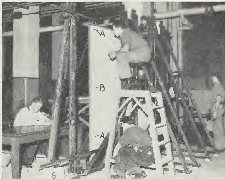
FIGURE 17.—Apparatus for racking load on specimen.
