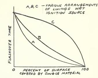
There is agreement between the one-third and the one scale when certain materials are used on the ceiling only. However, fiberboard is an exception being less dangerous on ceiling than on walls. Other materials are more dangerous on the ceiling. Flaming is generally observed below  $(\sim 4")$  rather than directly on ceiling surface.
