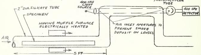
Variables which can be changed during the test include temperature of oven, velocity of oven along tube, and airflow rate. The photometer makes use of a photomultiplier tube and filter to correct for spectral sensitivity of the dark-adapted eye. It makes use of a 400 cps modulated light source and in this way changes in room illumination and flames do not affect results. This equipment has just been set up and it is still too early to report results.
