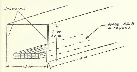
The tunnel is open at both ends and uses a wood crib as an ignition source. The time for flames to travel along the walls (which are lined with the specimen) and out the other end is measured.
