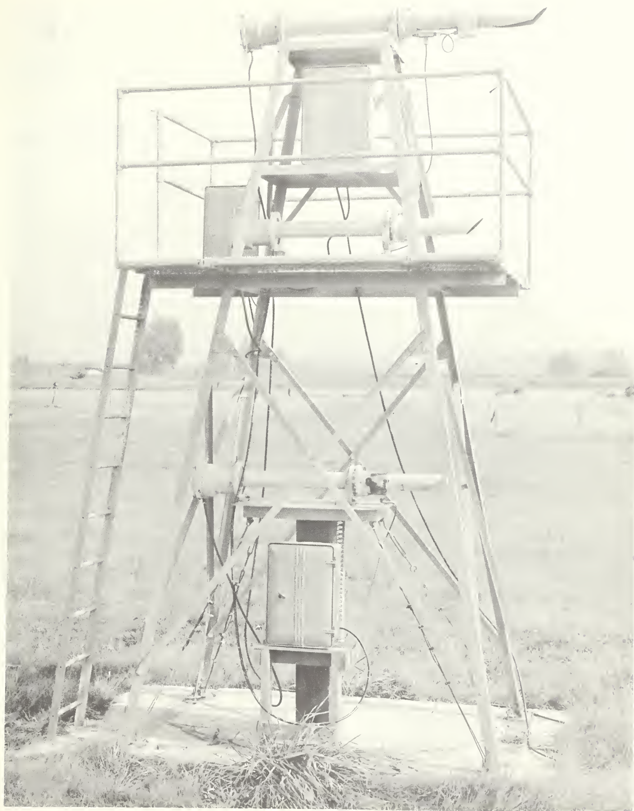
Figure 6. Transmissometer receiver installation to determine effect of height on transmission tests.
