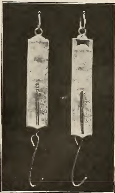
FIG. 61.— Straight-face spring scale with fraudulent sliding face
