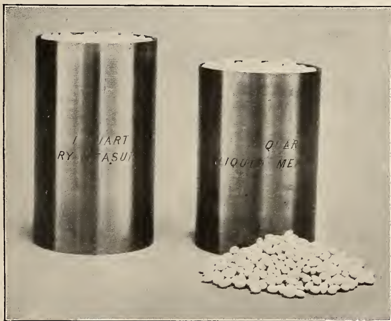
FIG. 10.— Comparison of deliveries of liquid quart and of dry quart
