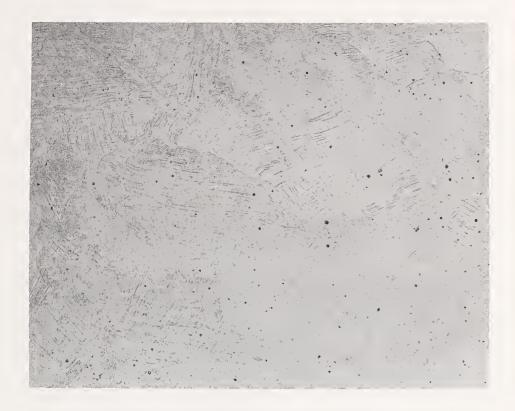
FIGURE I. Microstructure observed on a transverse surface after polishing and etching. Magnification 160X.
