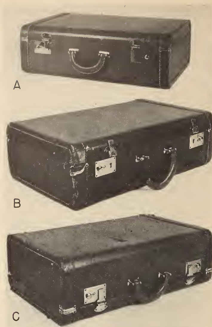
FIGURE 14. Small leather-covered case. A, Unused; B, after laboratory tests; C, after service tests.
