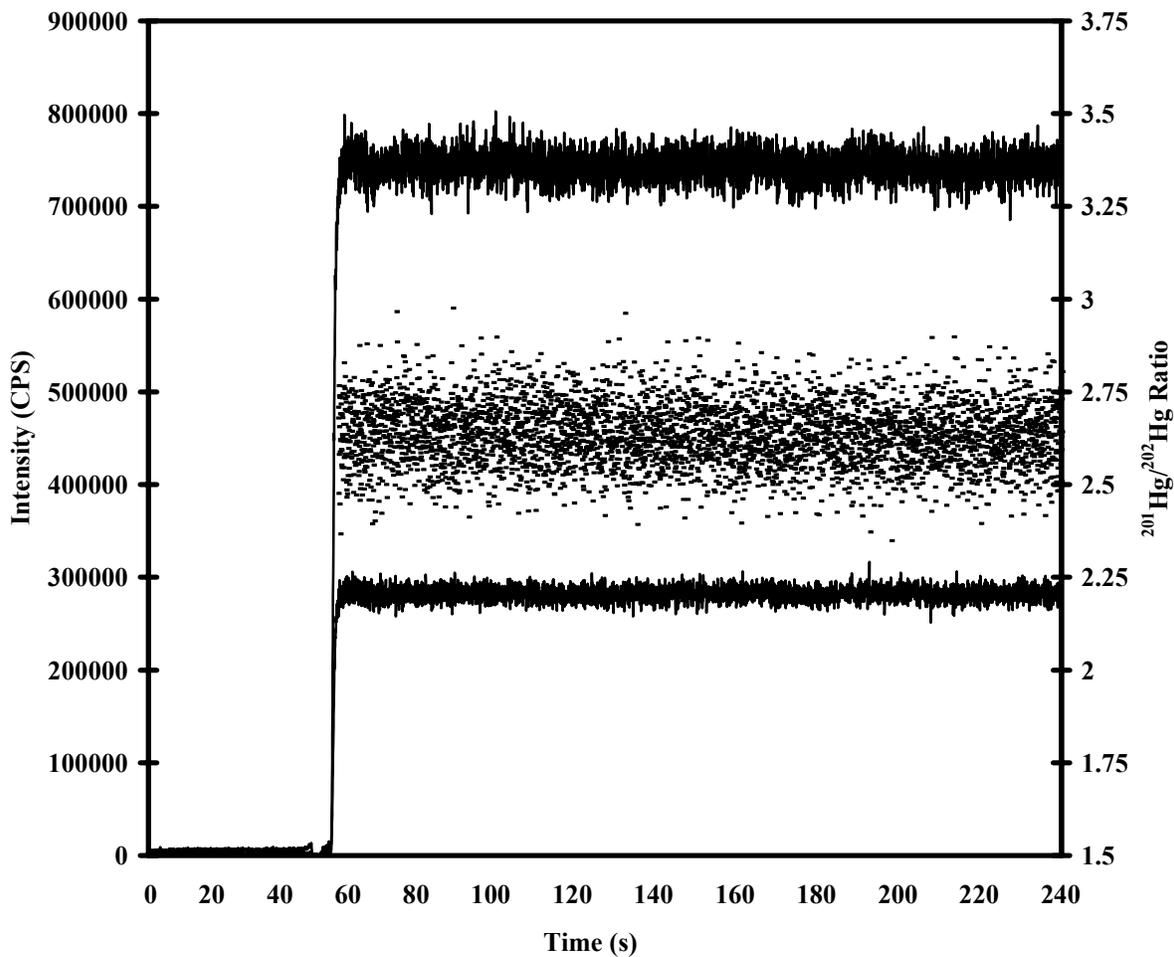
**Figure 2.** Transient profiles for  $^{201}\text{Hg}$  (top trace) and  $^{202}\text{Hg}$  (bottom trace) and overlay of corresponding  $^{201}\text{Hg}/^{202}\text{Hg}$  isotope ratio pairs for a  $^{201}\text{Hg}$  spiked common murre egg sample.
