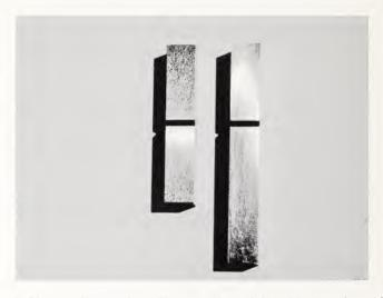
Figure 1. Photograph comparing a Charpy specimen (left) and Izod specimen (right).
