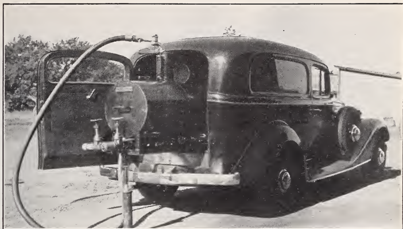
FIGURE 15.— Testing truck of the city of Springfield, Mass., showing test tank for measurement of large volumes of petroleum products.
