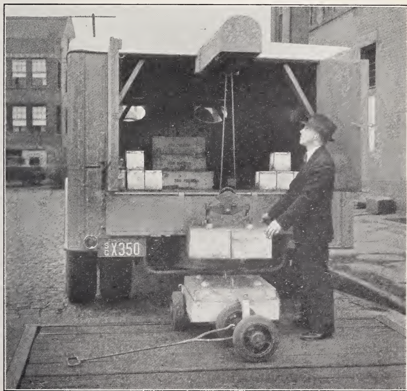
FIGURE 2.— Another view of New Jersey equipment showing crane, hoist, weight-handling truck, weights, and interior of body.
