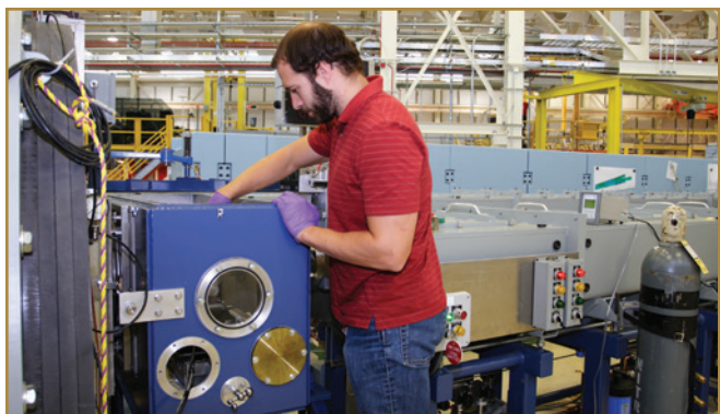
Dan Sunday (NIST MSED) carefully loads his samples into the sample chamber at NGB 10m SANS.
