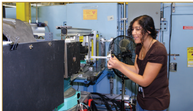
Natasha Khatri (Georgetown U) is mounting her molecular magnet sample for a polarized beam experiment at the NGD reflectometer.
