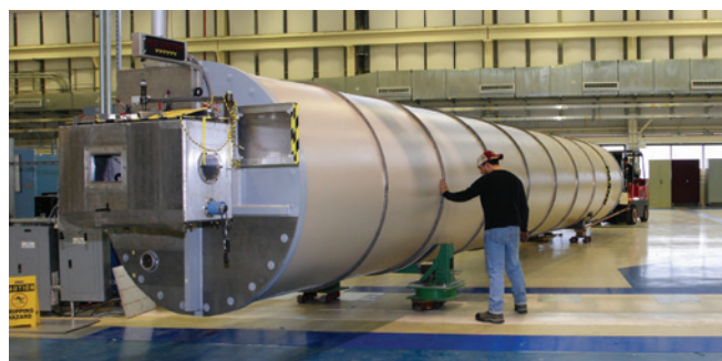
FIGURE 2: Riggers maneuver the 30 m SANS detector vessel from NG-3 to its new location on NG-Bu in the guide hall extension. (Photo credit: Yiming Qiu)
