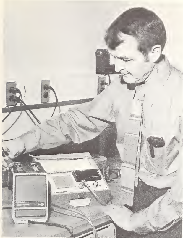
NBS-developed device testing the potential of heated surfaces to burn skin.
