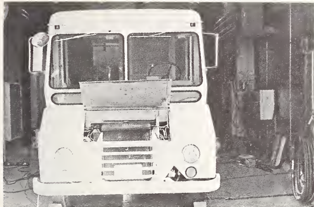
CNG-powered 1-ton Postal Service truck in NBS environmental chamber.
