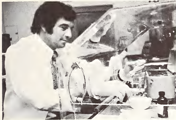
Mixing cement for hip implants under controlled conditions in incubator.
