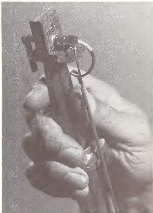
Device for measuring attenuation of high-frequency electrical signals.
