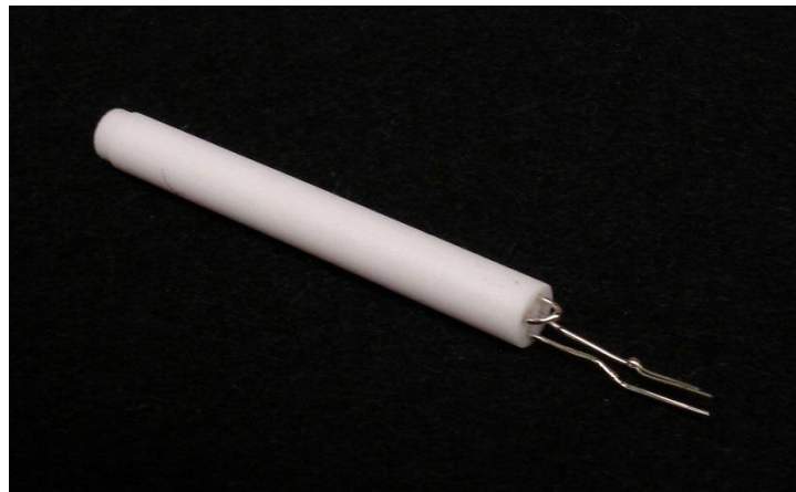
Figure 5. A completed resistor assembly from a 22 cm length of wire and a four-bore alumina insulator.
