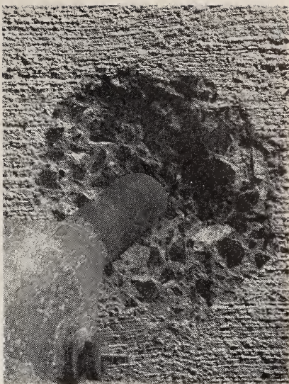
Left: Casting a specimen of experimental glass for measurement of its physical properties at high temperatures (p. 67). Right: Destructive action on concrete of hot gases at the temperature and velocity of the jet blast from aircraft. This was part of a study of concreting materials suitable as warmup, power check, and maintenance aprons for jet aircraft.
