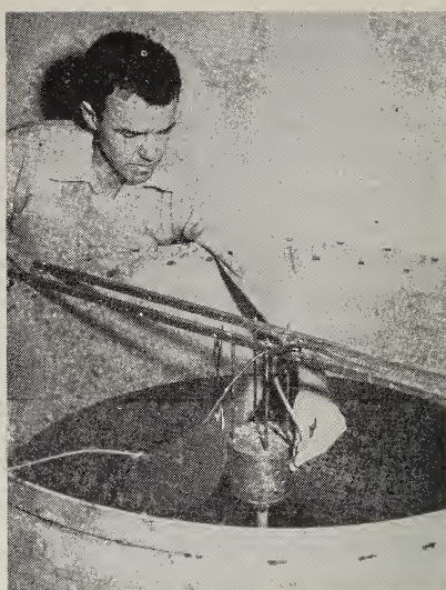
Methods of evaluating neutron sources. Left: An indium foil is inserted into pile containing neutron source; foil is later removed and its beta-ray activity measured. Right: A dip counter measures the activity of a manganese sulfate bath that has been irradiated by the national photoneutron standard. This permits calibration of the standard to within 2 percent (p. 36).
