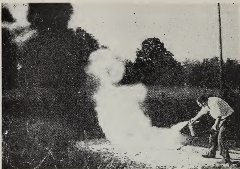
Application of a dry chemical extinguisher to a gasoline test fire. Extinguishing flammable-liquid fires by means of some types of dry powders has proved highly effective. Experiments indicate that only small quantities of the material are required (p. 73).
