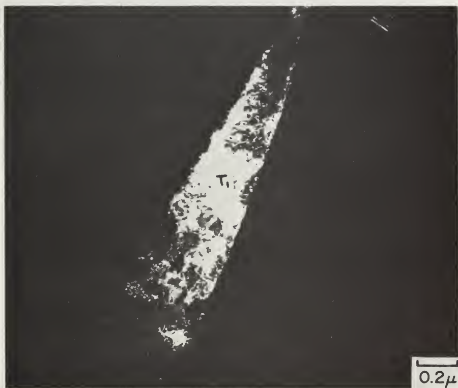
Fig. 28(b). Dark-field of T_1 employing twin reflection.
