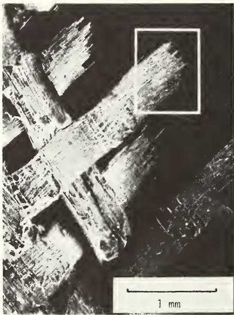
Fig. 2.4-K tensile failure, glass-polyimide.
