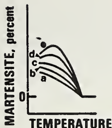
Fig. 5. Typical martensite-transformation-kinetics for Fe-18Cr-8Ni alloy on cooling below room temperature. The series of curves show the effect of progressively decreasing cooling rates, from (a) to (e).
