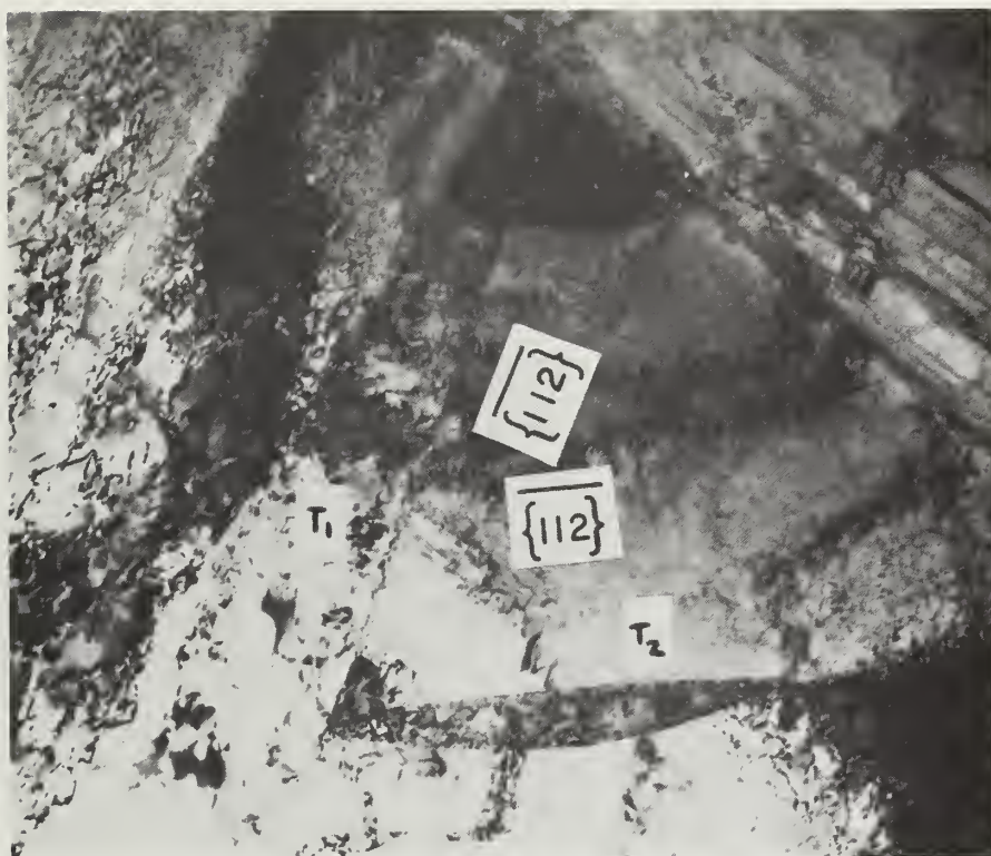
Fig. 28(a). Bright-field of twins T_1 and T_2 .
