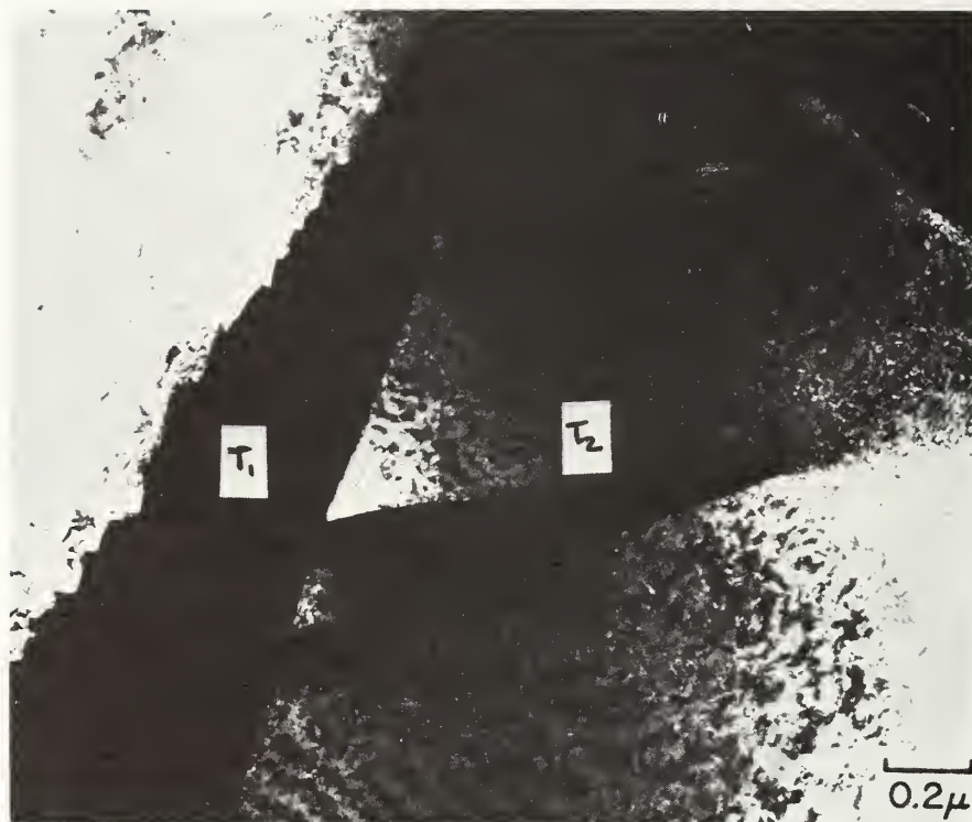
(c). Dark-field employing \delta matrix reflection.
