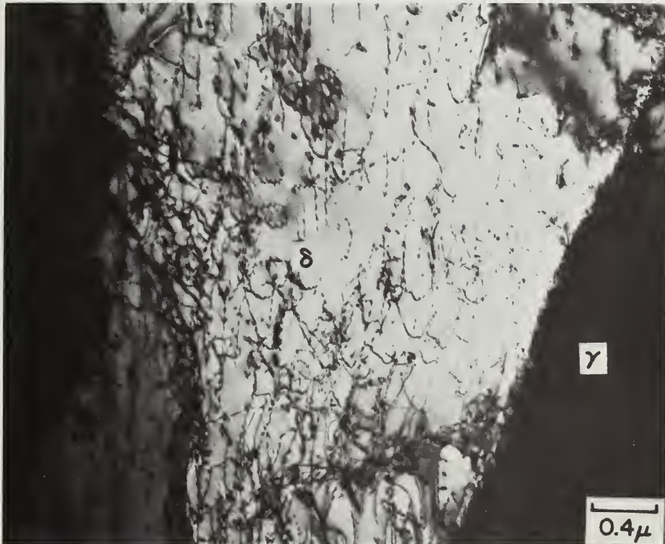
(c). 28.5 volume percent \delta , jogged dislocations and loops in \delta . Fig. 9. Dislocation debris. Transmission electron micrographs.
