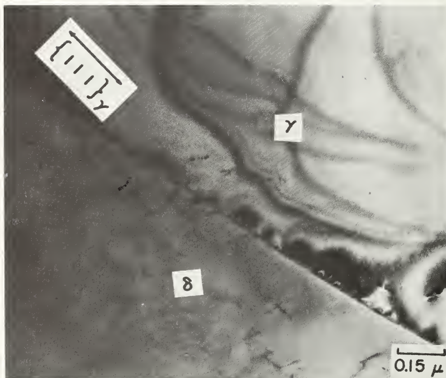
Fig. 10(a). 9 volume percent \delta , \delta/\gamma interface. Transmission electron micrograph.
