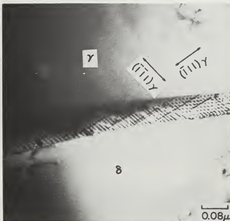
(b). Interfacial dislocation arrays.
