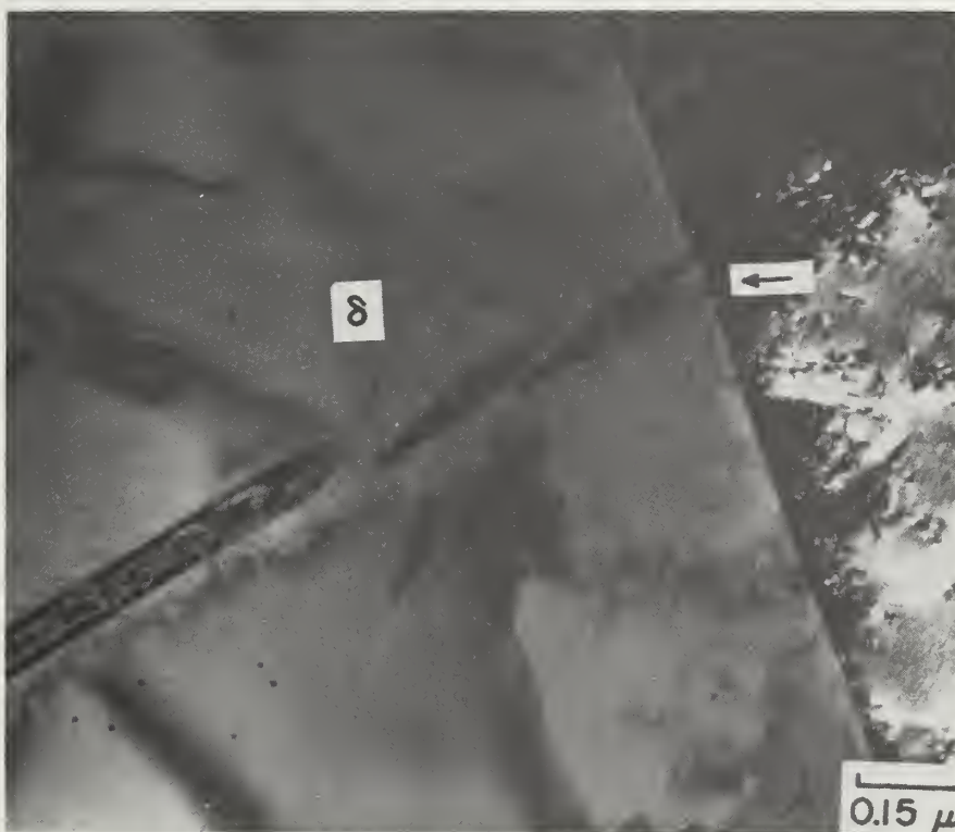
Fig. 23. 28.5 volume percent \delta , \epsilon=0.02 ; twin formation in \delta . Transmission electron micrograph.
