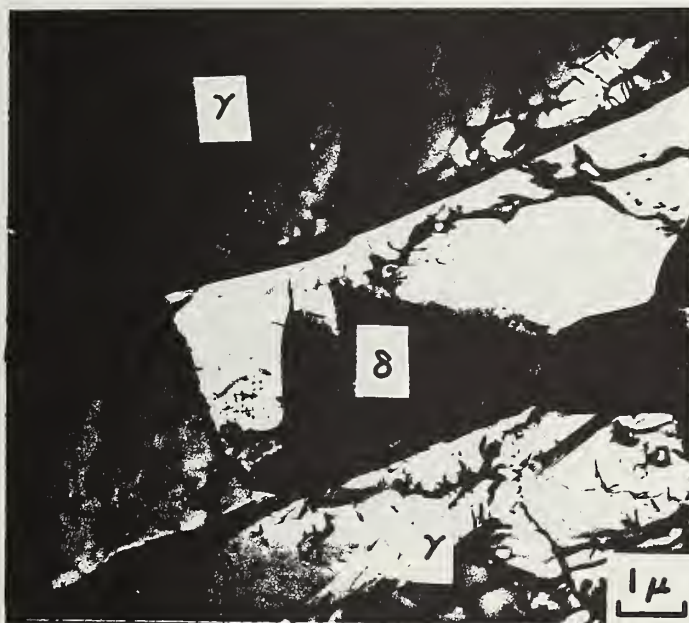
Figure 10 Recovered dislocation substructure in \delta , 28.5% \delta ; TEM.
