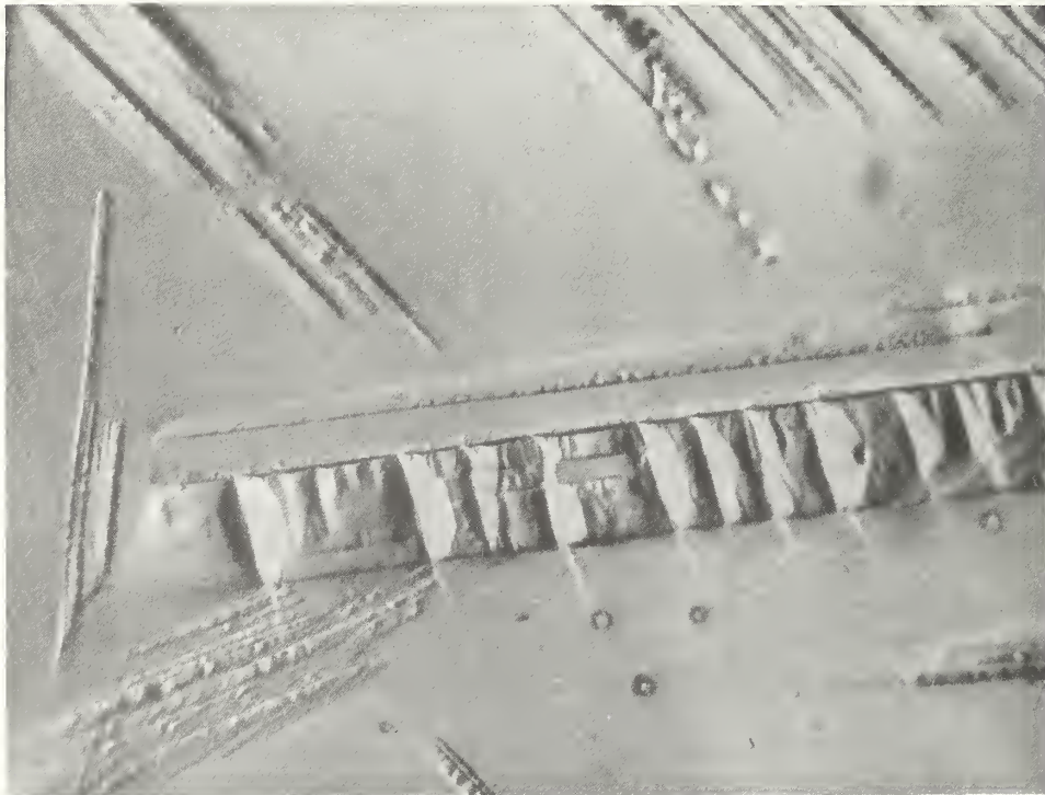
Fig. 9. (a) Shape deformation of martensitic transformation in austenitic stainless steel (Fe-Cr-Ni alloy, AISI 304L) on cooling to 76 K (230X). (b) Shape deformation of martensitic transformation in steel (AISI 304) flange previously used in service at 76 K (64X).
