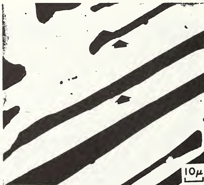
Figure 7 Residual \delta showing ledges on \delta/\gamma interface.
