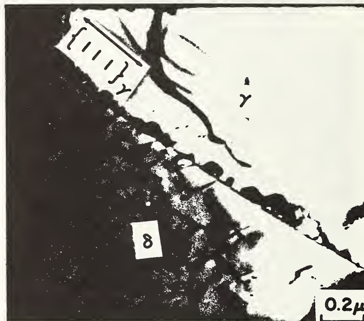
Figure 13(a) \delta/\gamma Interphase interface, TEM (a) BF
