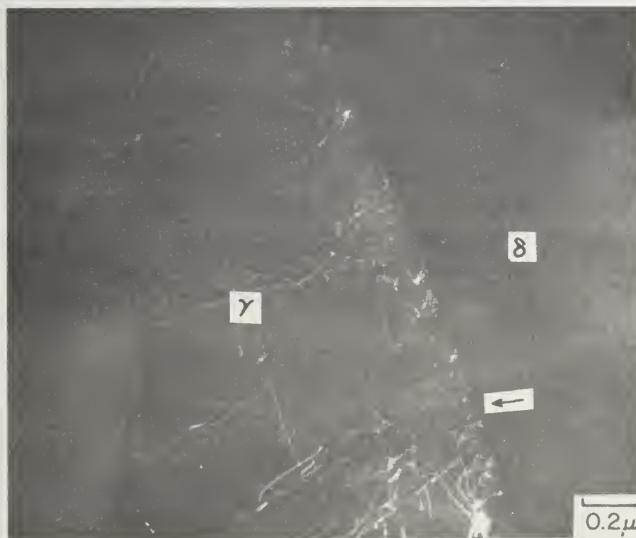
Fig. 13(c). 17.2 volume percent \delta ; bright-field and weak-beam dark-field.
