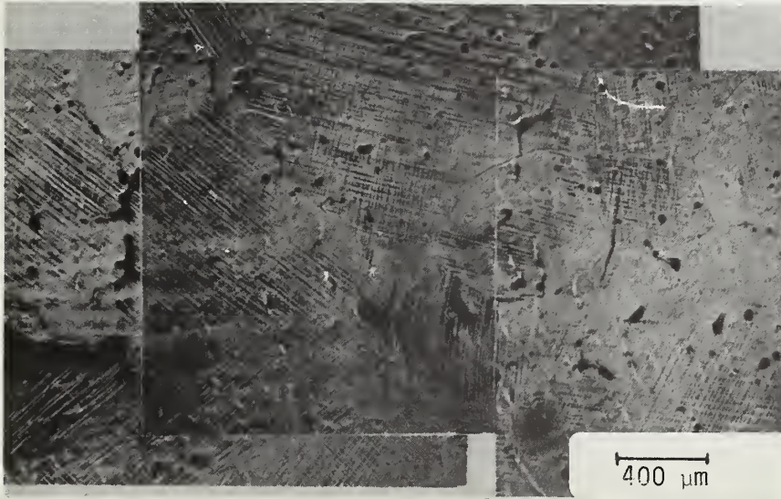
Figure 3. Area near the crack tip of a 0% delta-ferrite CF8 casting. Oxalic acid etch.
