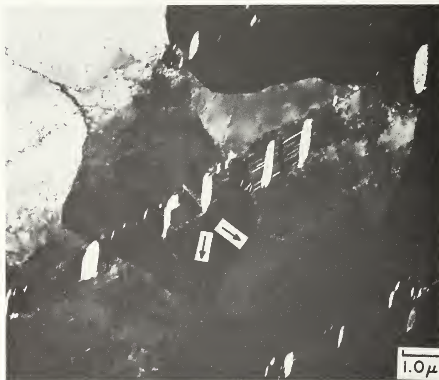
Fig. 21(b). Dark-field employing \alpha' reflection.
