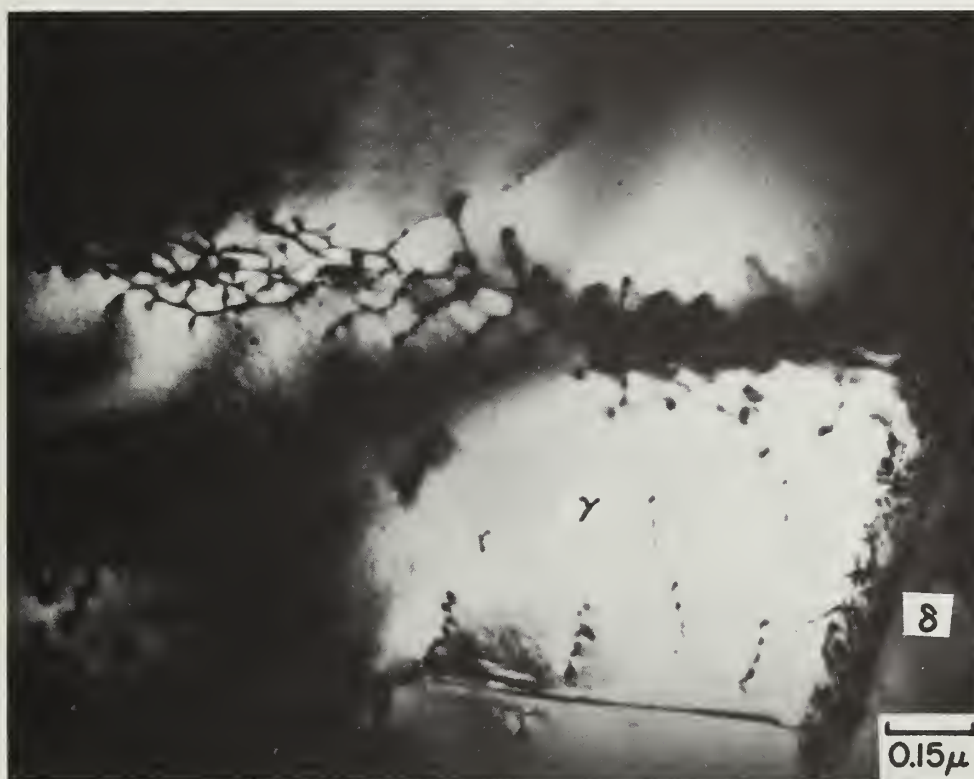
Fig. 8. 9 volume percent \delta , dislocation network attached to \delta/\gamma interface. Transmission electron micrograph.
