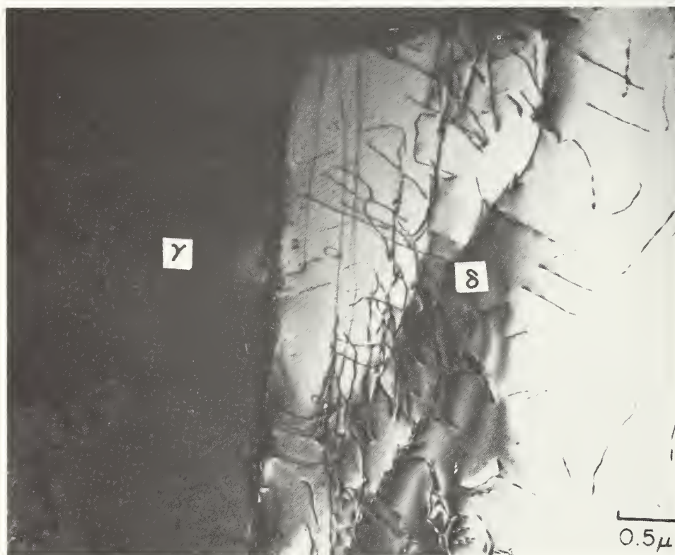
Fig. 9(b). 28.5 volume percent \delta , dislocations in \delta at \delta/\gamma interface.
