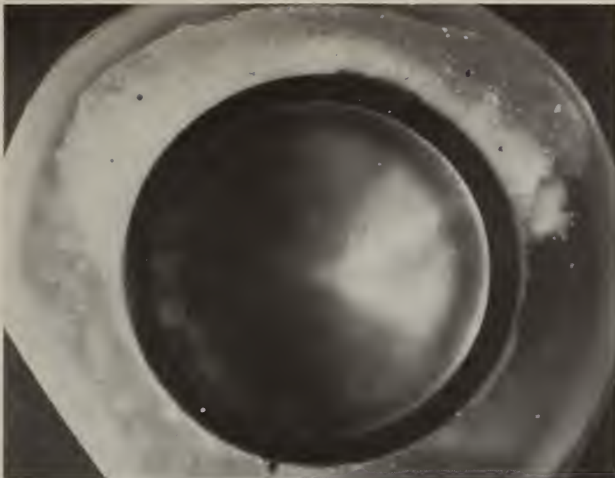
Figure 2. Section of Type 304 stainless steel tubing after exposure to K_2SO_4 seeded oxygen rich hot gas stream. Note formation of thick, 2 mm, deposit on upper surface. Tube temperature 500^{\circ}C . 6 X.
