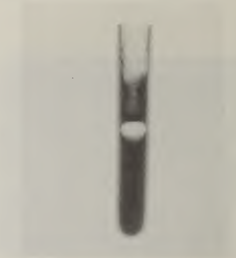
Figure 8 - Radiograph of crucible containing slag after being heated in an RF furnace to above the softening point. Note bubble formation.
