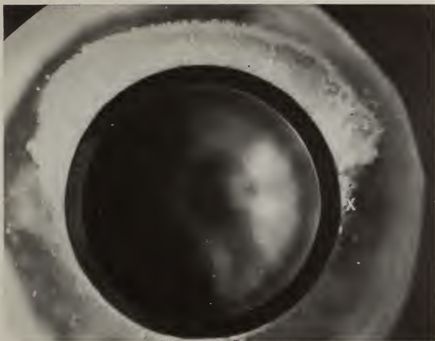
Figure 3. Section of Type 304 stainless steel tubing after exposure to K_2SO_4 seeded oxygen rich hot gas stream. Note formation of thick deposit on upper surface. Tube temperature 590^{\circ}C . 6 X.
