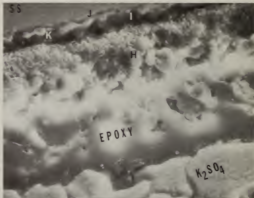
Figure 9. SEM micrograph, 1800 X, of reaction bands formed in the metal interface-columnar deposit powdery merge zone, location X of Figure 3. Lettered regions correspond to EDX spectra of Figures 10 and 11.
