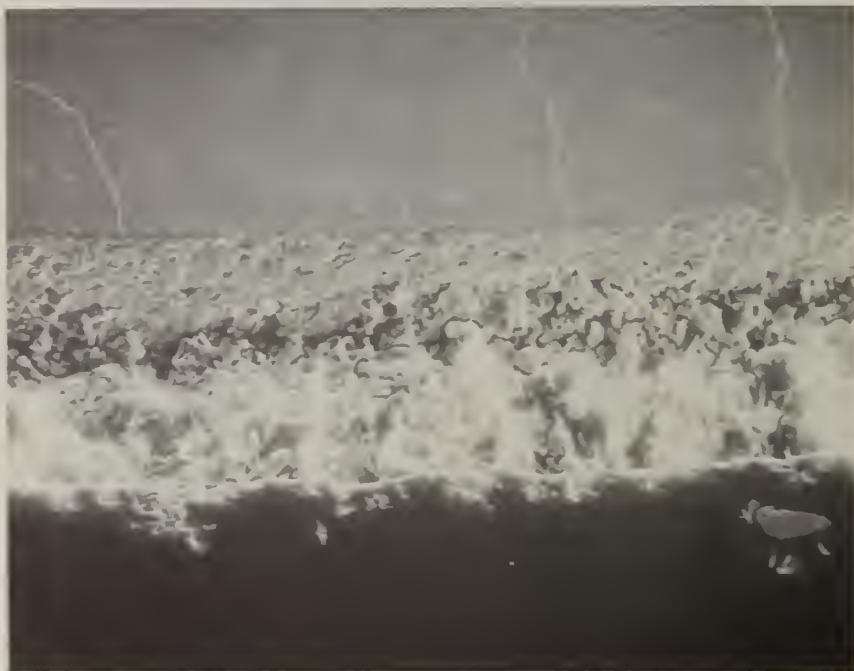
Figure 15. SEM micrograph, 190 X of reaction bands formed in the metal deposit interface of region Y of Figure 14.
