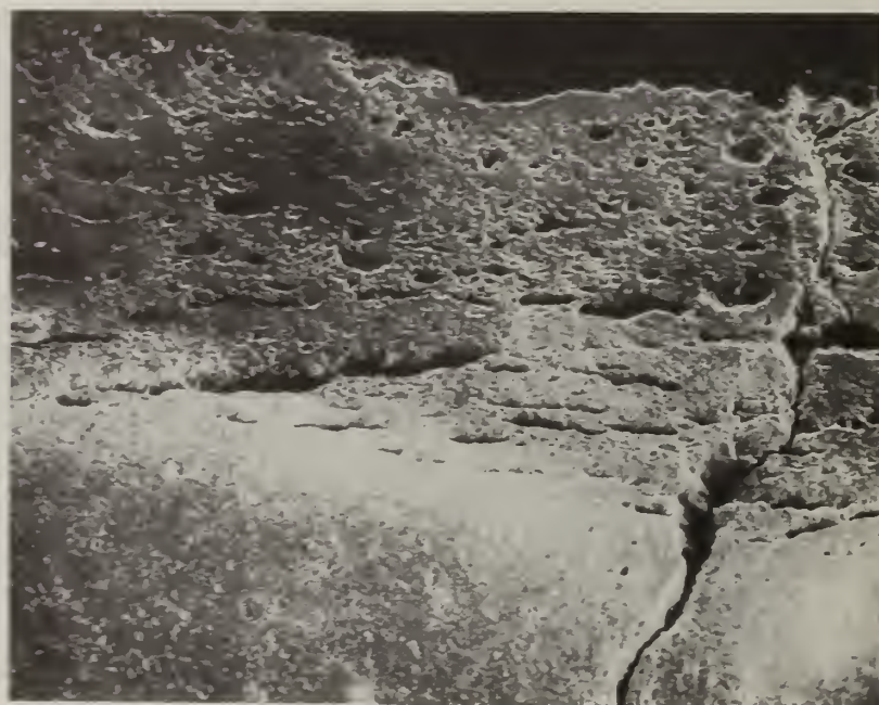
Figure 6 - Micrograph of cathode attack zone (upper half) of Bow NH slag with 20% K_2SO_4 added on YCrO_3 (.05 Mg). (40X)
