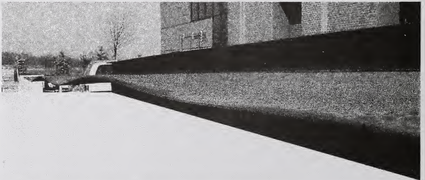
Figure 7 Photograph of 8' x 20' x 3/16" Plate - Severe Buckling
