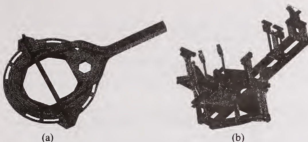
Fig. 3: FEA models for (a) weld product and (b) weld fixture.
