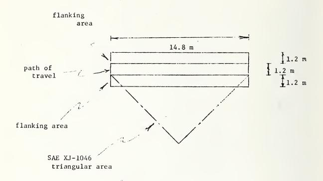
Figure 4. Measurement zones of SAE XJ-1046 and present procedure.
