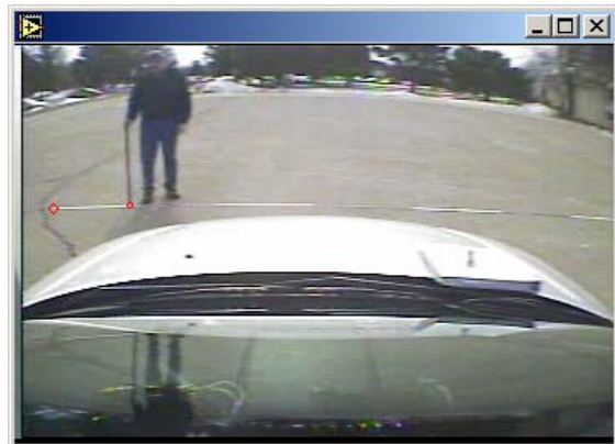
Figure 8. Forward camera calibration using one-meter sticks.
