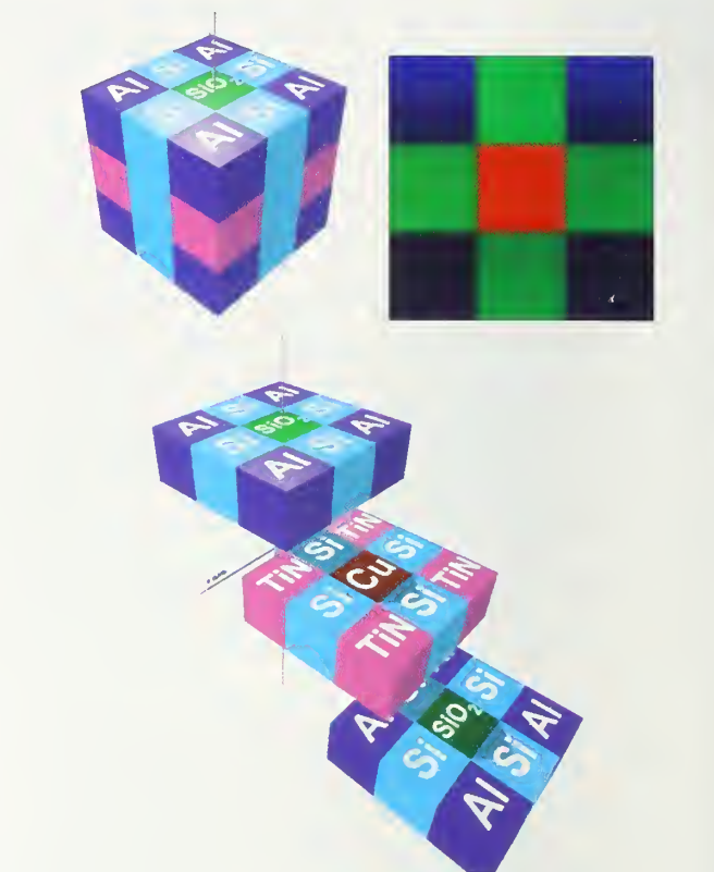
Figure 2. (top left) Phantom sample consisting of a "Rubik's cube" of aluminum, silicon, silicon dioxide, titanium nitride, and copper. This fictional sample contains many of the materials used in modern semiconductor devices, admixed and juxtaposed on the nanoscale to simulate the complexity of true 3D chemical imaging problems. Each of the 27 smaller cubes is 100 nm on an edge, so the entire assembly is 300 nm on an edge. The beam (purple vertical line) is shown striking the sample in the center of the \text{SiO}_2 subcube. (top right) 3-color X-ray elemental map showing quantitatively the detected X-ray intensities for the Cu K\alpha X-ray emission line (red), the Si K\alpha X-ray emission line (green), and the N K\alpha X-ray emission line (blue) after excitation with a 20 keV incident electron beam. Note the differential absorption of the Nitrogen K line from bottom to top (the X-ray detector is off the top of the image) and the bleeding of excitation near the phase boundaries. The X-ray map is 300 nm on a edge. (bottom) The same cube shown with the top, middle, and bottom layers vertically expanded and horizontally translated to reveal the 3D structure more clearly.
