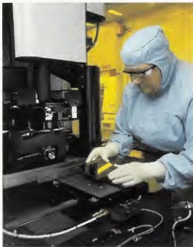
Figure 1. Maggie Crews inspects a mask generated in our optical pattern generator.
