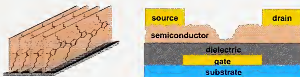
Figure 1. Schematic diagrams of the local structure of poly 3-hexylthiophene, an organic semiconductor near an interface (left) and the architecture for an organic transistor (right).
