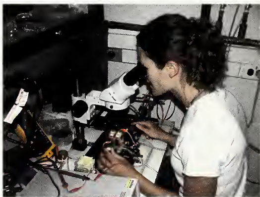
Figure 1. Elizabeth Mirowski characterizing spin-valve magnetic traps for microfluidic magnetic bead capture and sorting.
