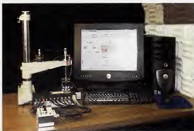
Figure 2. Fully automatic computerized nano-tip fabrication apparatus.
