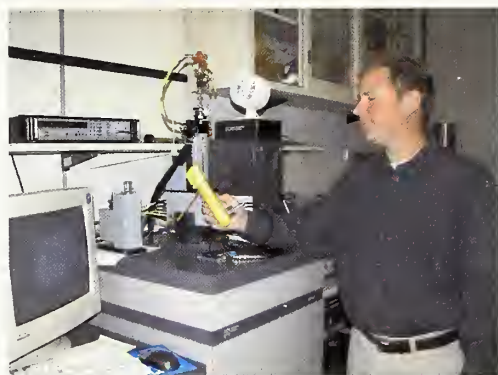
Figure 1. Brant Cage next to a magnetometer modified to simultaneously measure magnetic moment and high-frequency EPR spectra on nanomagnets.
