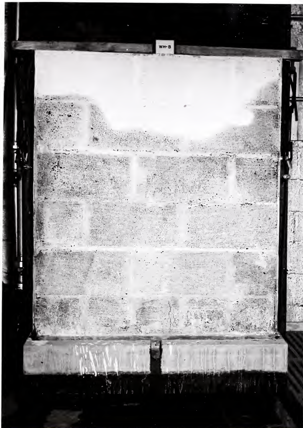
Fig. 8 - Back of wall B after test B-12. Holes drilled in top of exposed face, weep holes open, pressure head of 3-in.
