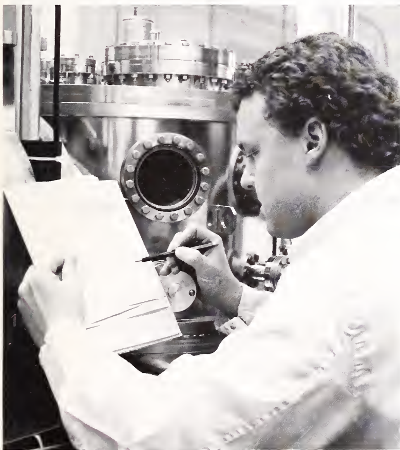
NIST physicist Todd Harvey observes sputter deposition of high-temperature superconducting thin films used by NIST to develop electronic measuring devices.
