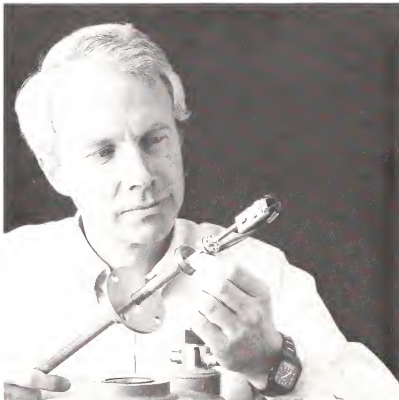
NIST electronics engineer Clark Hamilton examines the 1-volt Josephson series array voltage standard. With about 3,000 junctions, these NIST-fabricated integrated circuits are used in standards laboratories around the world.
