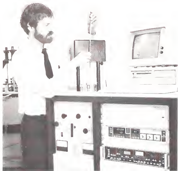
NIST physicist Ronald Goldfarb inserts a high-temperature sample into an ac susceptometer for magnetic measurements.
