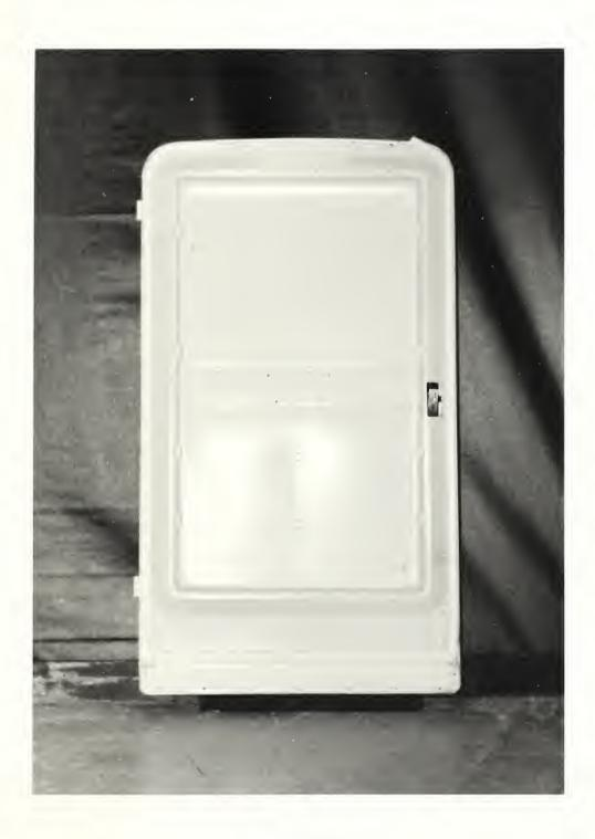
3. Adjustable Refrigeration Temperature control range. All four refrigerators tested held general food compartment temperatures well below 37°F in a 90°F ambient temperature as required but only the Westinghouse and Coldspot models could be adjusted to hold a temperature above 43°F. The Frigidaire and Admiral refrigerators failed this requirement, with general food compartment temperatures at the highest thermostat setting of 41.5°F and 38.9°F, respectively.
