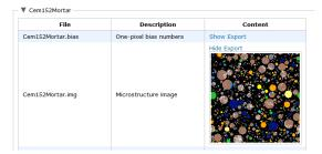
The thumbnail is a color image, with each color corresponding to a different phase in the mix. Once the thumbnail is displayed, it can be clicked with the mouse to open another page for more detailed examination and manipulation of the image.
