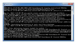
Warning: You must never close the Java console window during an active session of VCCTL. Doing so will cause VCCTL to terminate immediately and, in some cases, a portion of the database that keeps track of your running operations may also become corrupted. It is safest to simply minimize the console window to your desktop tray and leave it there while you are using VCCTL.
