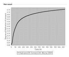
The plot is accompanied by a legend indicating both the hydration operation and the property, separated by a colon.
