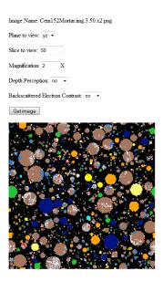
*Plane to view*: Choose one of three orthogonal directions from which to view the microstructure. The viewing planes are defined by the two Cartesian coordinate axes they contain (*e.g.*, the *yz*-plane is the plane observed when viewing along the *x*-axis).
