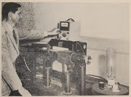
In an effort to extend and improve its temperature measuring capabilities, the Bureau developed this photoelectric pyrometer for temperatures above 1,000° C. Greater precision is possible than with the optical pyrometer presently in use (page 23).
