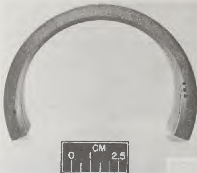
Figure 5. - Fabrication of cylinders by sputtering.
