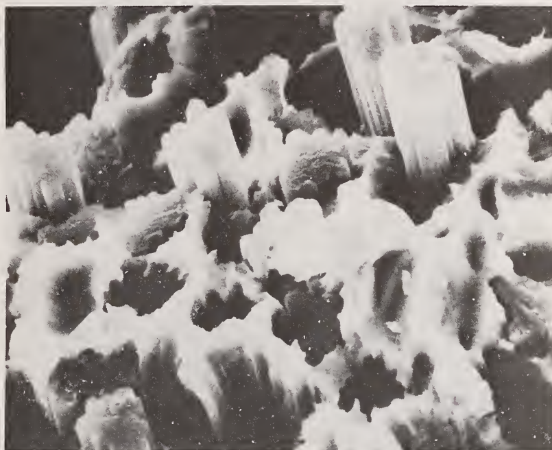
T50 (RAYON BASED)/A201 TENSILE FRACTURE SHOWING FIBER PULLOUT
