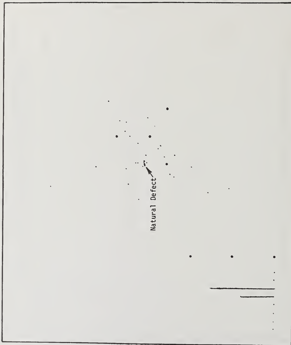
FIGURE 11. AE Sources Received from a Petrochemical Vessel Containing a 7.6 cm Crack - Early in Test
