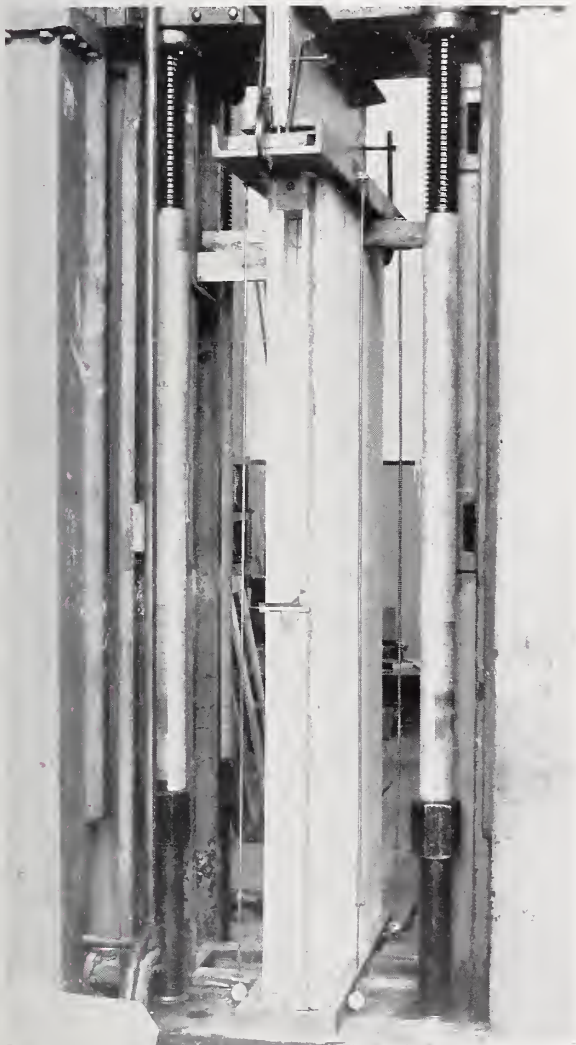
FIGURE 39.—Wall specimen BJ-C2 under compressive load.
