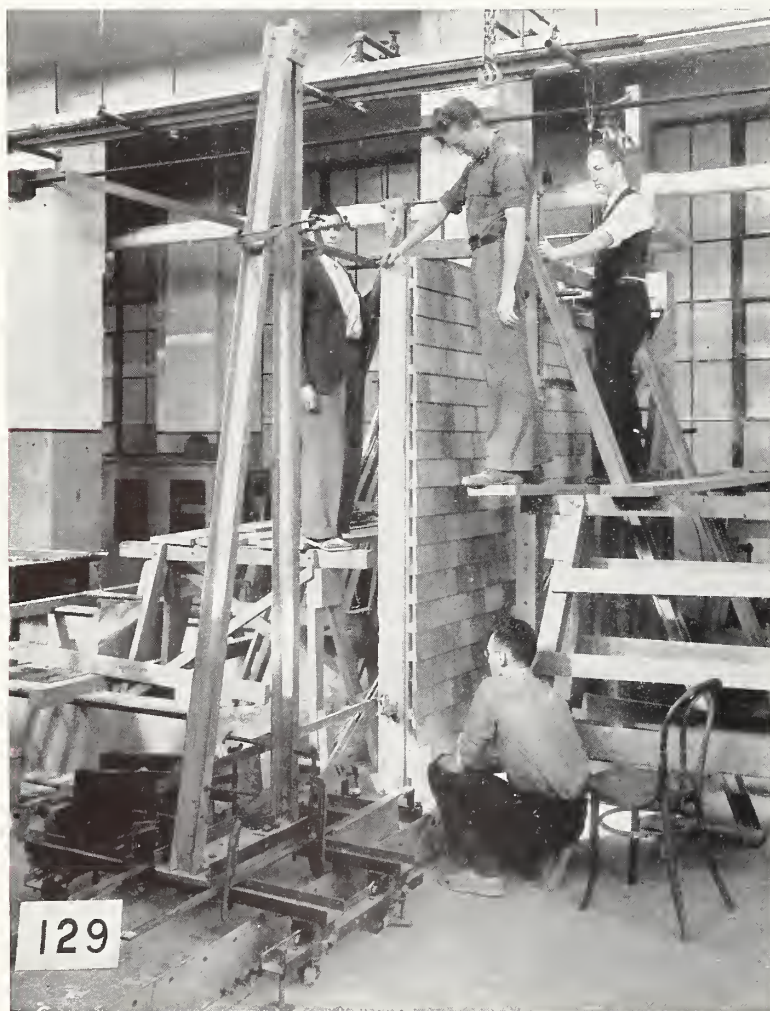
FIGURE 69.—Wall specimen BL-R1 under racking load.
