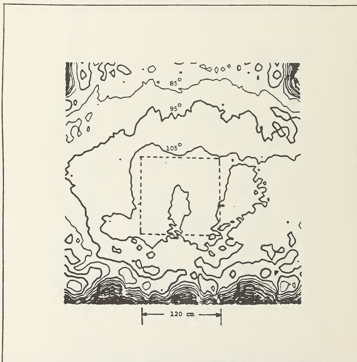
Figure 24. Compact range main component, 10^\circ phase contours, f = 18 GHz, horn probe.
