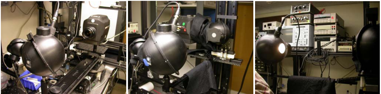
Figure 12. Apparatus used to provide an illuminance calibration of the integrating-sphere detector. Left picture shows the spectroradiometer measuring the exit port of the integrating-sphere source; middle and right pictures show the source being used to calibrate the integrating-sphere detector with its spectroradiometer.
