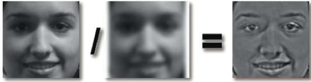
Fig. 7. This figure illustrates the computation of a self-quotient face image. The face image to the left is a cropped and geometrically normalized image. The image in the middle is the geometrically normalized image blurred by a Gaussian kernel. The image on the right is a self-quotient image. This image is obtained by pixel-wise division of the normalized image by the blurred image.
