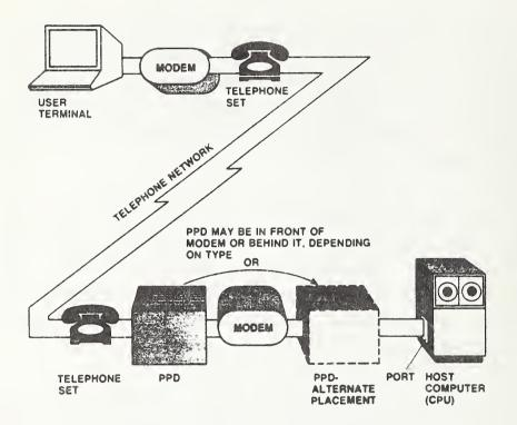
Figure 6-1 Dial-Up Circuit -- With Host Port Protection
