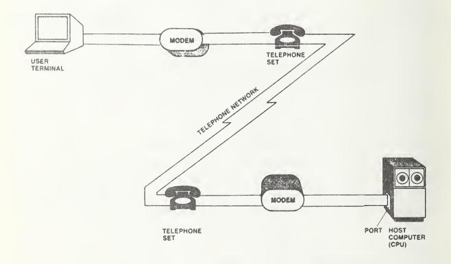
Figure 2-2 Dial-up Circuit -- Normal Configuration
