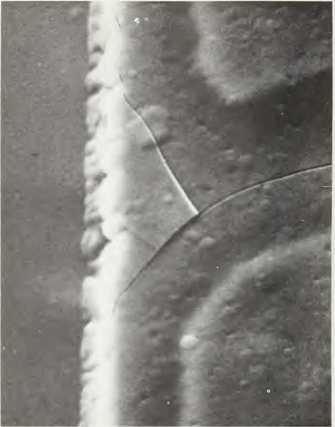
Figure 11. Scanning electron micrograph (4800X, 30°) showing a different area of sample from figure 10. Gray channel areas are caused by differences in charging due to etched-out aluminum under glass.
