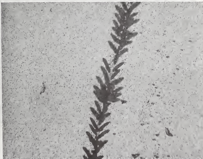
Figure 4. Scratch-induced microcracks in glass layer similar to figure 3. Most damage occurs in V-shaped part of pattern. Maximum spread of demarcation is 80 \mu\text{m} (385X, brightfield).
