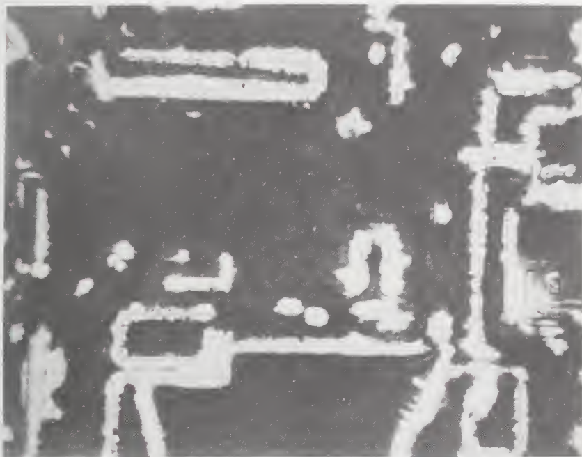
Figure 40. Carbon black deposited on device to reverse-decorate the defects. High contrast renders microscopic evaluation fast and sensitive. Width of narrowest aluminum lines (visible at right) is about 12\text{ }\mu\text{m} (150X).
