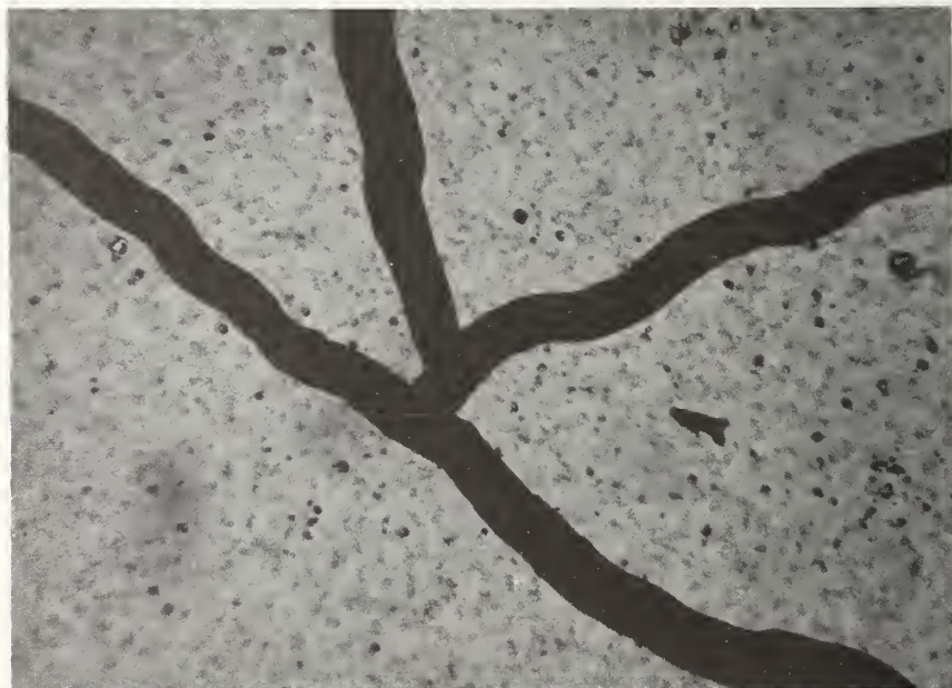
Figure 2. Etching-demarcated microcracks in sample shown in figure 1. Dark bands are substrate from which aluminum was removed from underneath glass layer in 10 min selective metal etching at 50°C. Glass crack is dark line in center of 15-18- \mu\text{m} -wide bands. No pinholes are present in this sample area (385X, Nomarski differential interference contrast).
