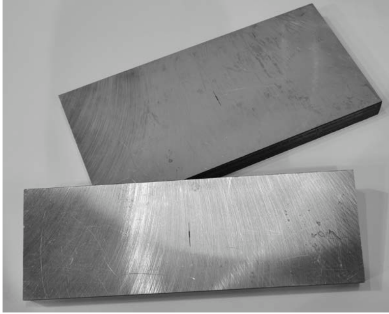
Figure 9 – Flat-plate reference standard development specimens in the EDM notched condition.
