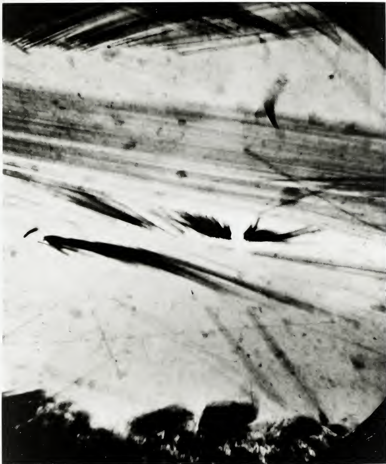
FIGURE 9. GLASS FIBER REINFORCED CLAY EMULSION ON A COATED BASE SHEET
