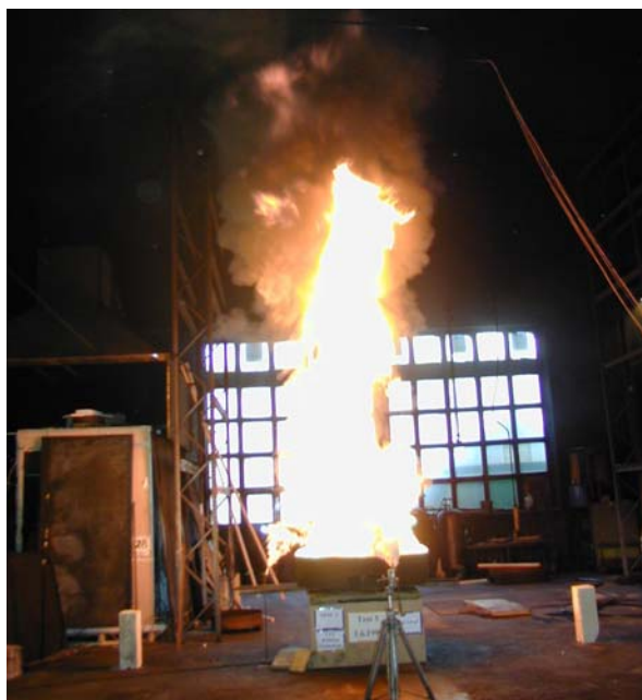
Figure A-22. Photographs of Heptane Pan Fires, VTT Large Hall Tests, Case 2 (Courtesy, Simo Hostikka, VTT Building and Transport, Espoo, Finland)
