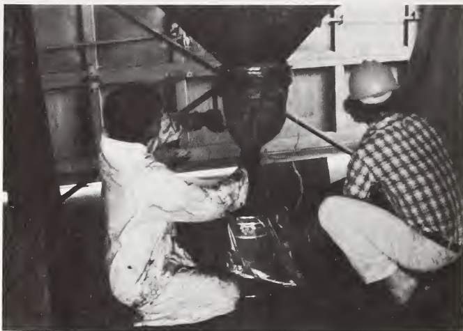
Figure 8. Closing Flow from Blender During Filling of 5-Gallon Pails
