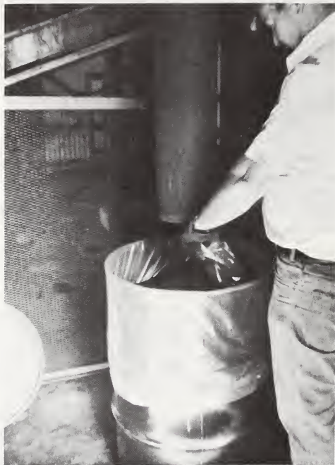
Figure C-4. Collection of Coal Sample and Companion 5000 Gram Sulfur Analysis Sample at Delta Mine
