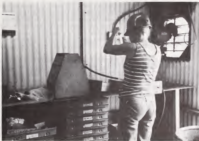
Figure C-7. Air Cleaning of Laboratory Pulverizer.
