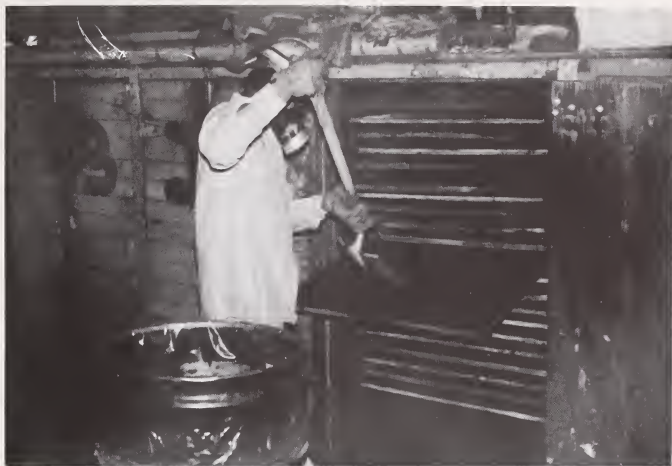
Figure 2. Tray Loading and Oven Drying of Coal Sample
