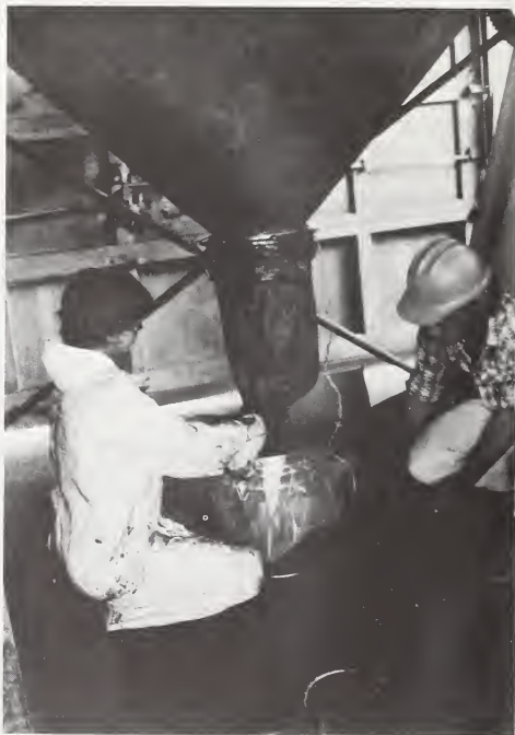
Figure 7. Discharging of Blended Coal into Lined 5-Gallon Pails
