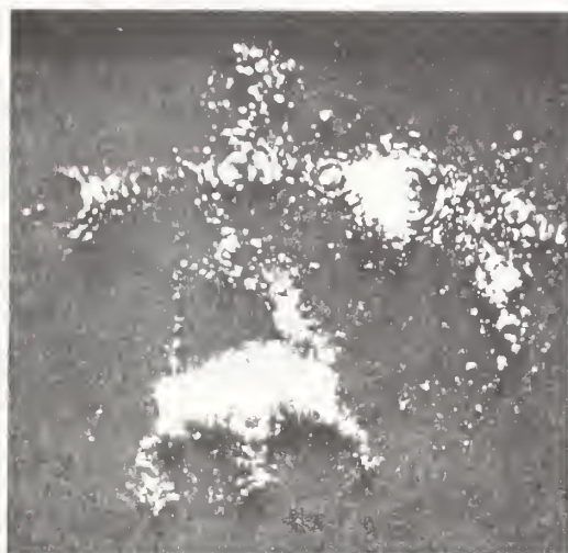
Fig. 14. A neon field ion micrograph obtained from uranium, 30K, 15,500 volts.
