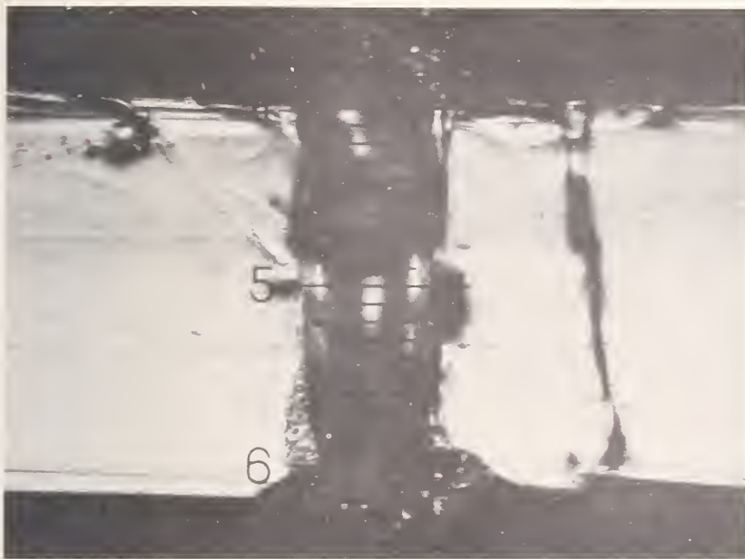
Cross section photograph of a failed transistor sliced in half shows the perforation (large vertical dark region) which forms a short circuit between the emitter (top) and the collector (bottom). (Small divisions of comparison scale through middle of view are approximately 0.00035 inch.) Recent NBS transistor failure studies have clarified the mechanisms of such breakdowns. (See p. 127.)
