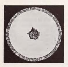
Figure 2. Overall view of SRM 480 showing the alloy wire at center encased in pure Mo (white) and pure W at the outer rim. X10
