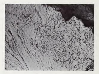
Figure 1. Micrograph of the heavily etched alloy wire. Note highly strained material and absence of inclusions and voids. Interface between Mo and the alloy wire is at upper right. X1000
