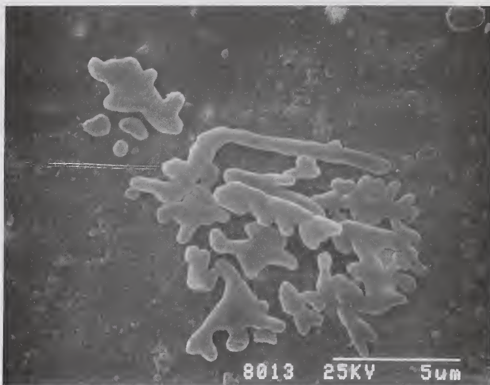
Figure 11.9 0° Tilt SEM Photomicrographs of Flat from 1 % Dimethy-n-Octadecylchlorosilane in PPO Lubricated \text{Si}_3\text{N}_4 BTF Test at 60 kg: a) Exit Region, b) Exit Region (Higher Magnification)
