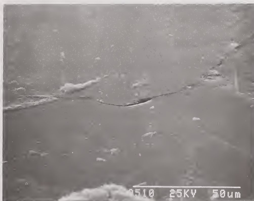
Figure 10.27 SEM Photomicrograph of Wear Scar on Pin from PPO Lubricated POD Test on Fused Silica: a) Wear Scar, b) Higher Magnification of Radial and Tensile Cracks outside Wear Scar
