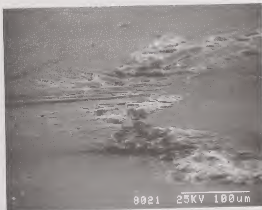
Figure 11.7 75° Tilt SEM Photomicrographs of Flat from 1% Dimethy-n-Octadecylchlorosilane in PPO Lubricated \text{Si}_3\text{N}_4 BTF Test at 60 kg: a) Wear Scar, b) Entrance Region
