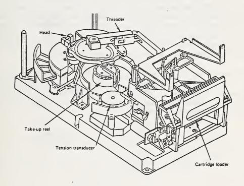
Figure 3. 3480 Type Tape Drive Assembly.
