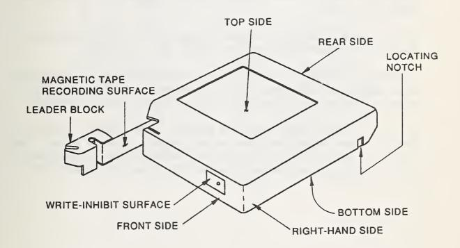
Figure 2. 3480 Type Tape Cartridge Assembly.
