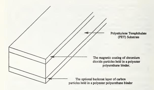
Figure 1. 3480 Type Tape Structure.
