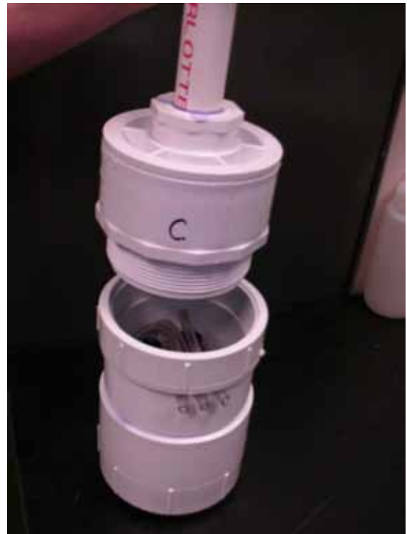
Figure 6. Diagram (A) and photograph (B) of the gas sampler used to collect stream samples for gas analysis in the reaeration study on Tacony/Frankford Creek, Philadelphia, Pa., 2009. (Photograph by Andrew Reif, U.S. Geological Survey)
