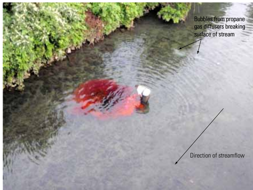
Figure 5. Dye injection and propane gas diffusion on September 3, 2009, in Tacony/Frankford Creek near U.S. Route 1, Philadelphia, Pa. (Photograph by Jason Cruz, Philadelphia Water Department, on September 3, 2009.)
